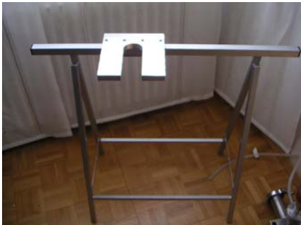
Reactor holder, with the base-plate where the Reactor may hang.
