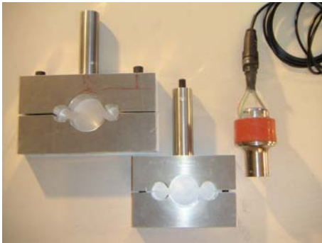
Different Clamp-on elements and high power MMM converters.
