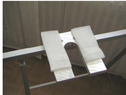
Reactor holder with foam-type backing in order to avoid direct metal-to-metal contact between the Clamp element and the holder base-plate
