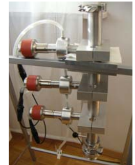
Reactor placed on the holder. Different possibilities for mounting are presented.
