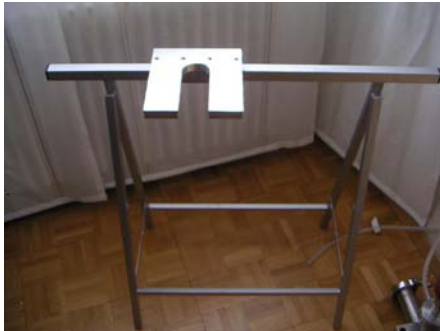
Reactor holder, with the base-plate where reactor should hang.
