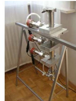
Reactor placed on the holder. Different possibilities for mounting are presented.
