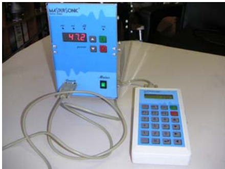
Handheld controlled generator with MSH-1 controller unit
